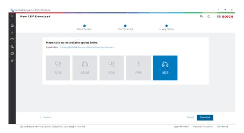
The downloaded data will be stored in \\Documents\Bosch\Crash Data Retrieval 2 folder with <\mathcal{VIN-number>\_<ecu-name>.cdrnx} if VIN input is available from user during the download; otherwise the file name will be <17 - (hyphens)>\_<ecu-name>.cdrnx. Here the ecu name is ACM or ADS based on the ECU from which the CDR data is downloaded.
